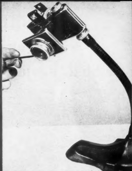
A gooseneck desk lamp makes a fine adjustable tripod for table top work if the socket is removed and a \frac{1}{4} "x20 bolt fitted to engage the camera.
